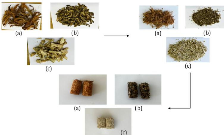
Raw agriculture waste materials used in the study: (a) coconut fiber, (b) groundnut shell (c) sugarcane fiber.
