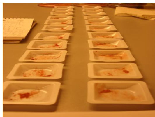
Fig. 1. Modified Devonian clay - Na modified and Ca modified for sorption kinetics tests at Linnaeus University laboratory
