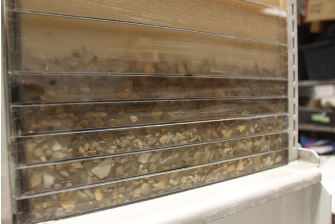
Fig. 6. Separating limestone and oil shale with minijig
