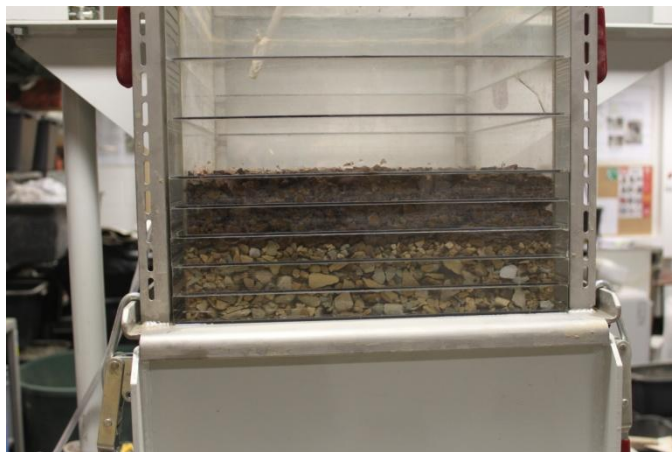
Fig 7. Separated material inside the minijig sample box before removal
