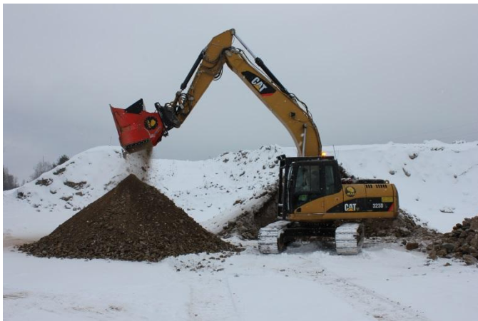
Fig. 3. ALLU crushing bucket test in Narva open cast
